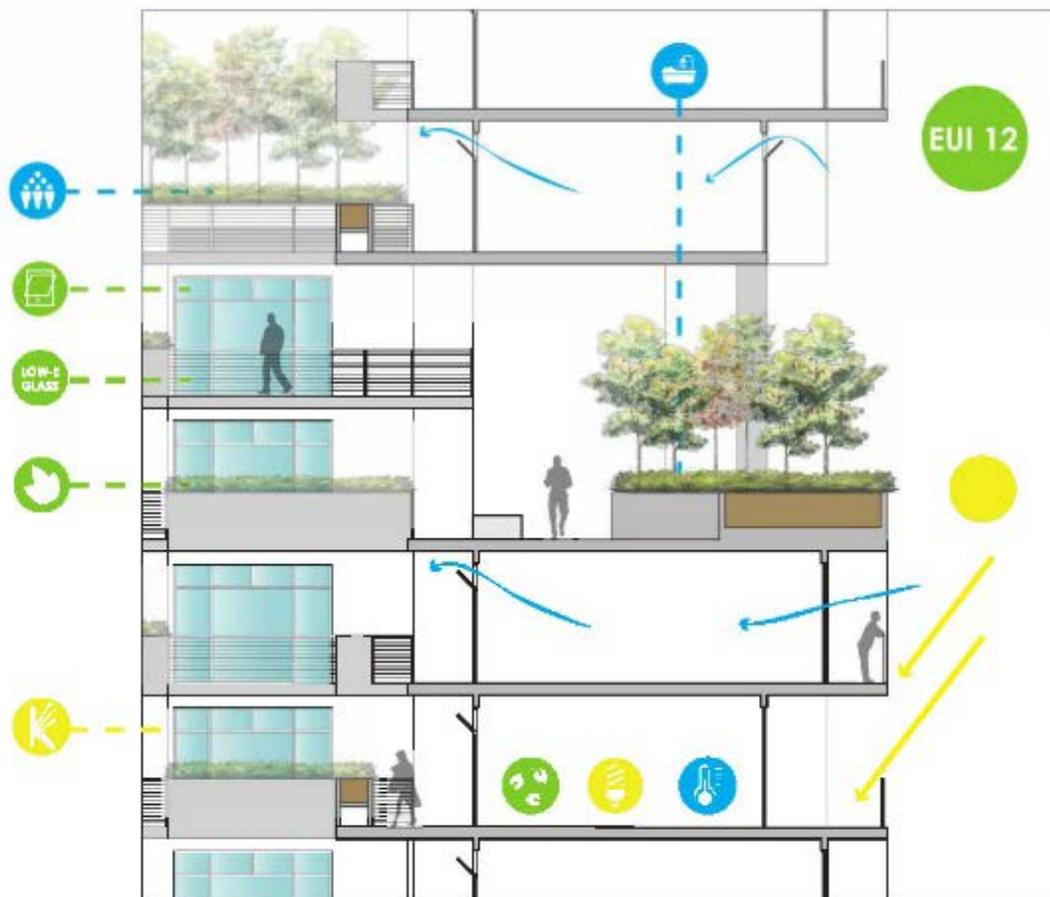
Passive heating was also implemented and the simplest method to passively heat a building is to increase solar gains to the interior of the building through direct gain systems.
